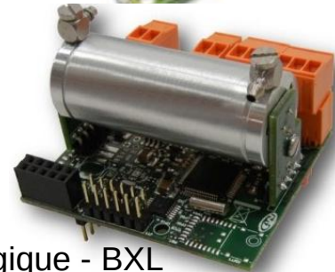
Figure 1. The CORA device used for monitoring CO 2 concentrations in cave air. The yellow box underneath the device holds eight 1.5 V batteries (D cells).
