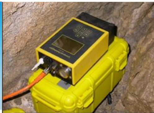
Figure 1. The CORA device used for monitoring CO 2 concentrations in cave air. The yellow box underneath the device holds eight 1.5 V batteries (D cells).
